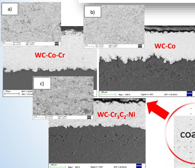
Figure 1. Cross-section and microstructure of manufactured coatings: a) WC-Co-Cr, b) WC-Co, c) WC-Cr<sub>3</sub>C<sub>2</sub>-Ni
