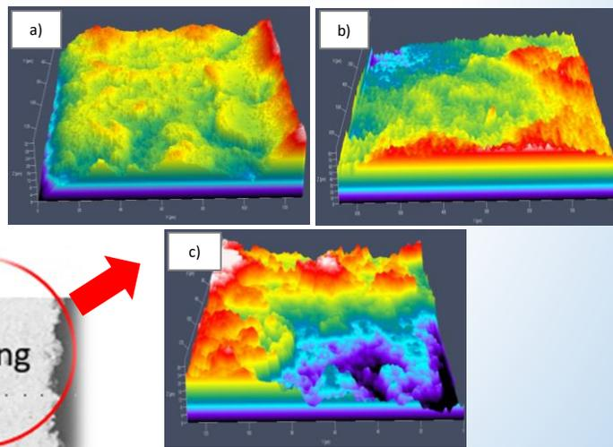
Figure 2. The topography of manufactured coatings: a) WC-Co-Cr, b) WC-Co, c) WC-Cr<sub>3</sub>C<sub>2</sub>-Ni
