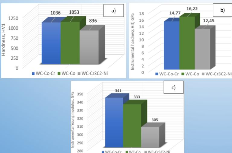
Figure 3. Comparison of: a) hardness HV1, b) instrumental hardness HIT, c) instrumental Young modulus EIT
